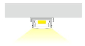
Extrusion can be mounted to benches, cabinets, shelves or furniture with the use of Velcro tape or mounting bracket.
