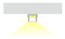
Extrusion can be mounted to benches, cabinets, shelves or furniture with the use of Velcro tape or mounting bracket.
