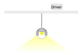
Extrusion can work as a pendant for over desk or bench top applications with the use of suspension kits.
