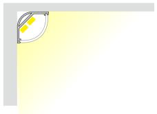
Extrusion is perfect for the joints between walls, cabinets or ceilings with the use of double-sided tape or mounting brackets.
