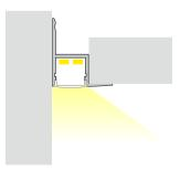
Extrusion can be recessed into benches, cabinets, shelves or furniture with the use of mounting bracket.
