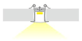
Extrusion can be recessed into benches, cabinets, shelves or furniture with the use of double-sided tape or mounting glue.
