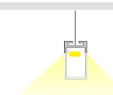
Extrusion can work as a pendant for over desk or bench top applications with the use of suspension
