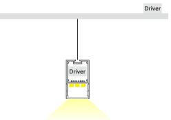
Extrusion can work as a pendant for over desk or bench top applications with the use of suspension kits.
