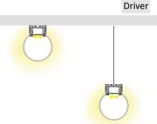
Extrusion can work as a pendant for over desk or bench top applications with the use of suspension kits.
