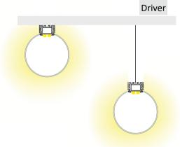
Extrusion can work as a pendant for over desk or bench top applications with the use of suspension kits.
