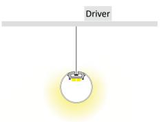
Extrusion can work as a pendant for over desk or bench top applications with the use of suspension kits.
