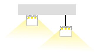
Extrusion can work as a pendant for over desk or bench top applications with the use of suspension kits.
