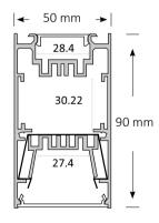
Extrusion can be surface mounted to ceilings with brackets or suspended using suspension kits.
