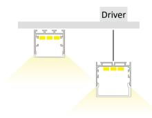
Extrusion can be surface mounted to ceilings with brackets or suspended using suspension kits.
