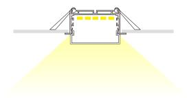
Extrusion can be recessed into ceilings or walls with the use of mounting clips.
