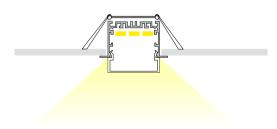
Extrusion can be recessed into ceilings or walls with the use of mounting clips.
