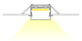
Extrusion can be recessed into benches. cabinets, shelves or furniture with the use of mounting clips.
