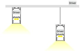
Extrusion can be surface mounted to ceilings with brackets or suspended using suspension kits.
