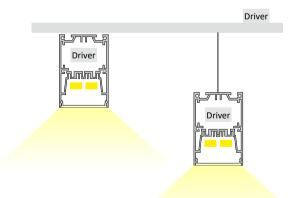
Extrusion can be surface mounted to ceilings with brackets or suspended using suspension kits.
