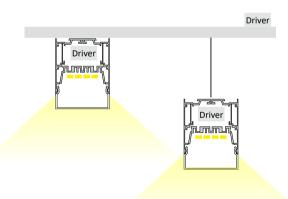
Extrusion can be surface mounted to ceilings with brackets or suspended using suspension kits.
