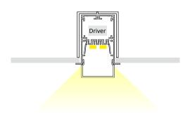
Extrusion can be recessed into ceilings or walls with the use of mounting clips.
