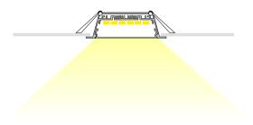
Extrusion can be recessed into ceilings or walls with the use of mounting clips.
