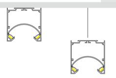
Extrusion is suitable for surface mounted and suspended applications, where limited glare is a requirement.
