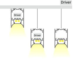
Extrusion can be surface mounted to ceilings with brackets or suspended using suspension kits.
