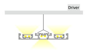
Extrusion can work as a pendant for over desk or bench top applications with the use of suspension
